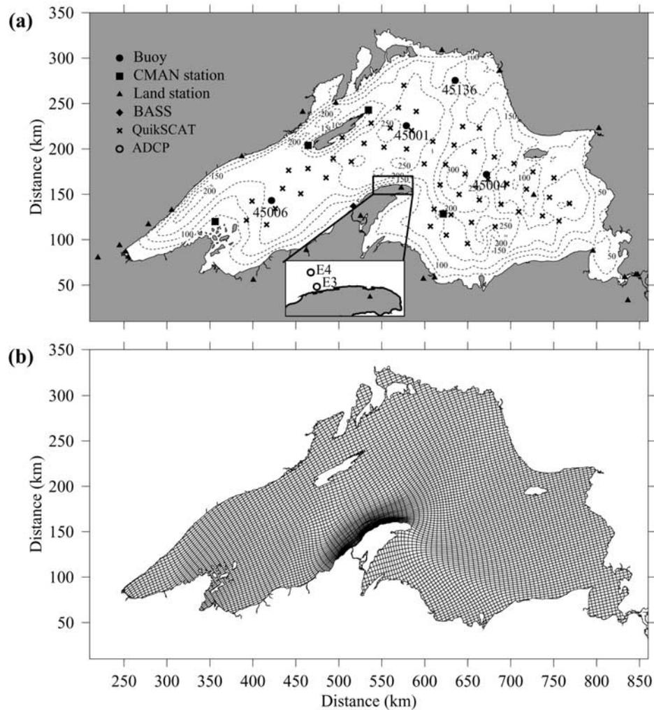
**Figure 1.** (a) Bathymetry (in meters) and locations of buoy, QuikSCAT, and other meteorological measurement stations and bottom-mounted tripods and ADCP sites over and around Lake Superior as well as (b) the nonorthogonal grids of the Lake Superior model. Solid and dashed lines in Figure 1a indicate the contours of the isobath in meters, and E3 and E4 shown in the box enclosed by heavy solid lines are the locations of the bottom-mounted ADCPs.
