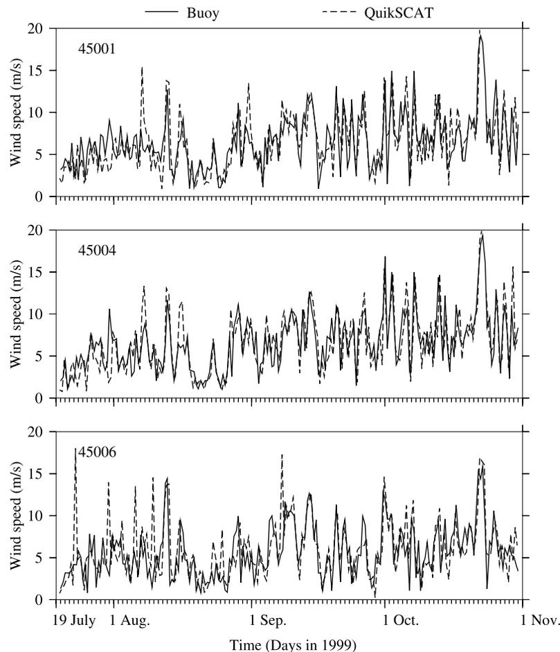
**Figure 2.** Comparison of the time series of the surface wind speed measured on buoys and QuikSCAT at buoys 45001, 45004, and 45006 for 19 July to 31 October 1999. The figure was replotted using the data shown by Haddock and Ralph (submitted manuscript, 2003).
