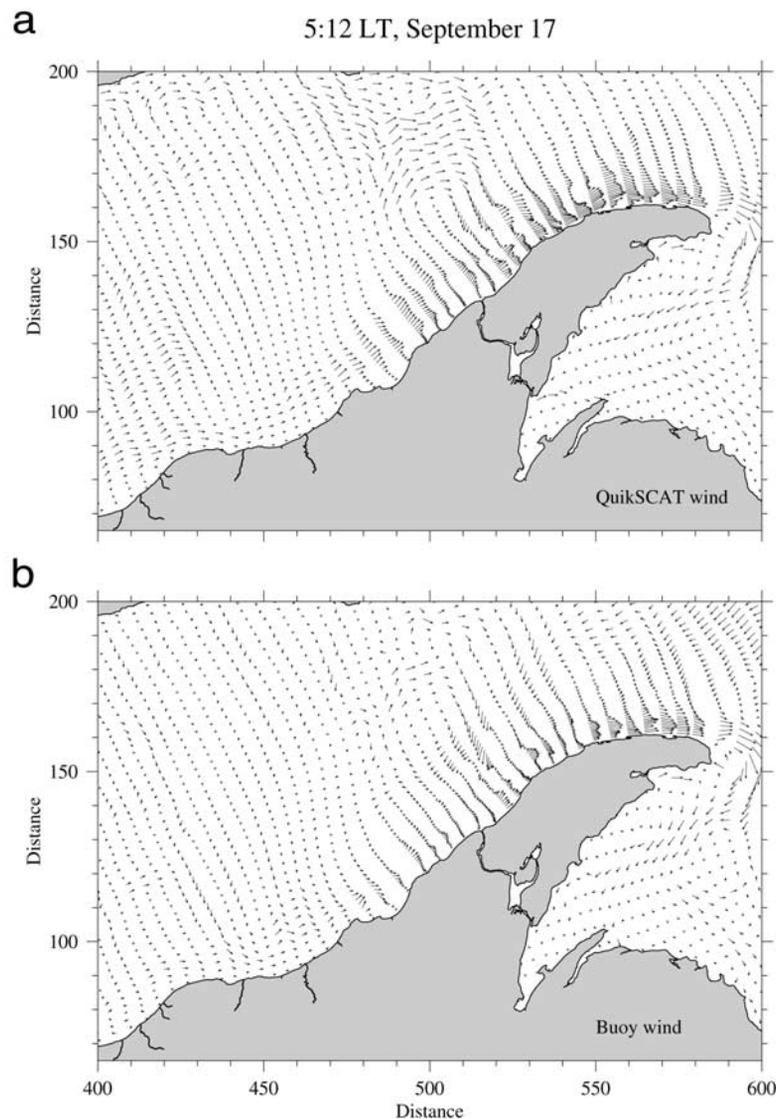
**Figure 8.** Distribution of surface water current vectors predicted at 0512 LT on 17 September by the model runs with (a) QuikSCAT and (b) buoy winds, respectively.
