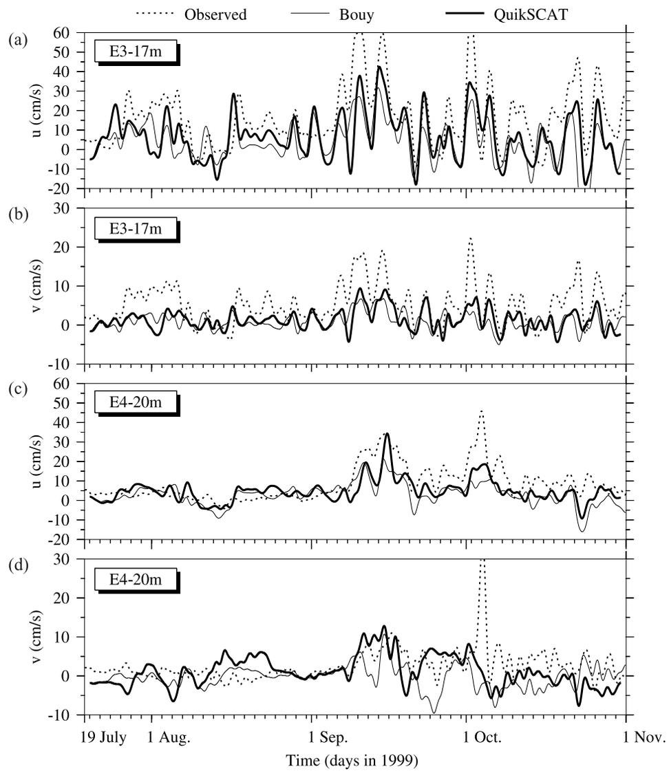
**Figure 9.** Comparison of observed and model-predicted water currents at depths of 17 and 20 m at site E3 and E4 for 19 July to 31 October 1999.
