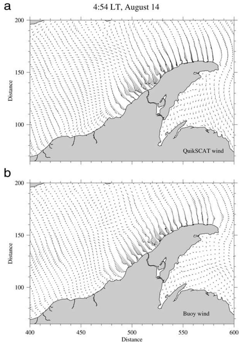
**Figure 7.** Distribution of surface water current vectors predicted at 0454 LT on 14 August by the model runs with (a) QuikSCAT and (b) buoy winds, respectively.
