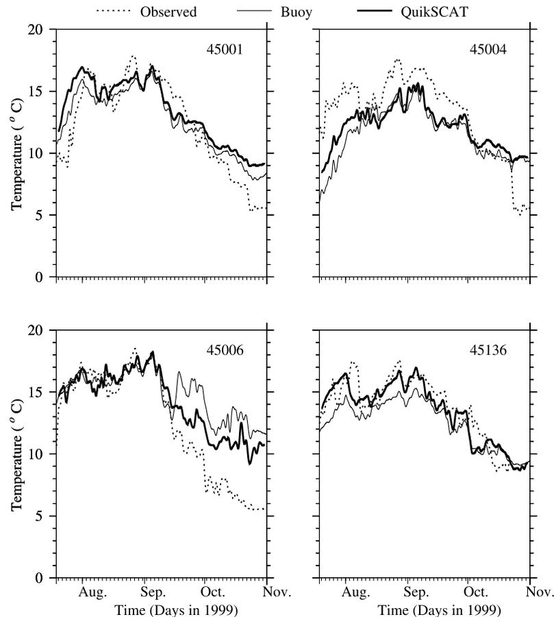
**Figure 3.** Comparison of the temporal variation trends of surface water temperatures observed on buoys and predicted by the model runs with the buoy and QuikSCAT winds on buoys 45001, 45004, 45006, and 45136 for 19 July to 31 October 1999.
