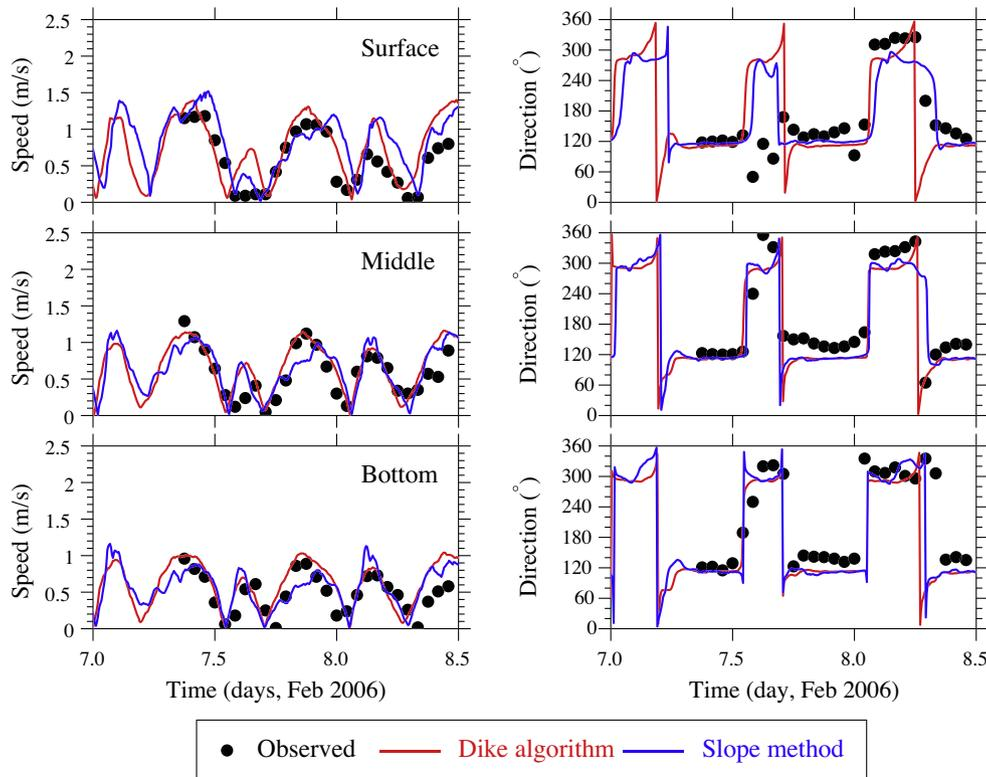
**Fig. 17.** Model-data comparisons of current velocity (left) and direction (right) during February 2006 at the surface (upper), mid-depth (middle) and near bottom (lower). The solid black dots indicate the field data. The blue and red lines indicate the results with the dike–groyne algorithm and bed-comforting slope method, respectively. (For interpretation of the references to color in this figure legend, the reader is referred to the web version of this article.)
