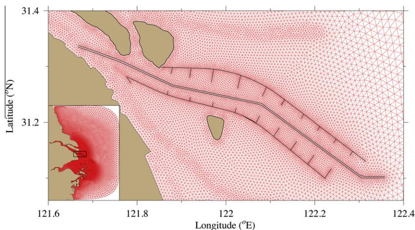
**Fig. 14.** Enlarged view of the triangular mesh with dikes and groynes around the Deepway Channel off the Changjiang. The panel inserted in the lower left corner shows the computational domain and mesh of the local domain FVCOM with inclusion of the Changjiang, Hangzhou Bay and the inner shelf of the East China Sea.
