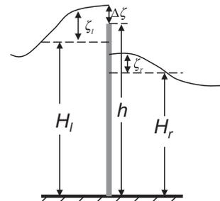
Fig. 3. Illustration of the treatment of the water exchange across a dike or a groyne when the water on either side is over the height of the construction.
