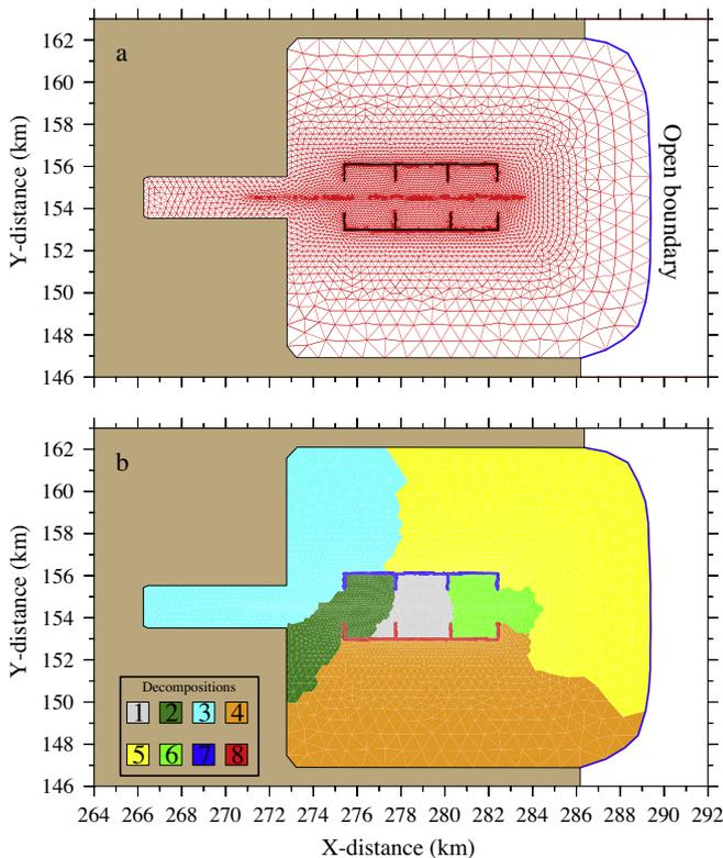
**Fig. 9.** The computational domain and unstructured triangular mesh (a) and domain decomposition (b) for the idealized estuary case. Bold solid lines inside the domain are the dikes and groynes specified in the model.
