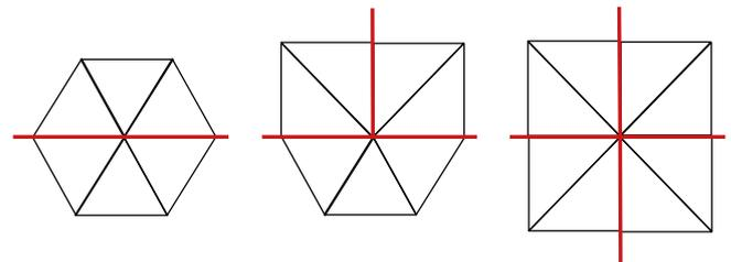
**Fig. 1.** Three types of dike and groyne construction. Type 1: a straight dike (left panel). Type 2: a groyne joined at its end with a dike (middle panel). Type 3: a groyne crossed through a dike (right panel). A horizontal red line indicates a dike and a vertical red line represents a groyne. The black lines are the triangle's edges. (For interpretation of the references to color in this figure legend, the reader is referred to the web version of this article.)
