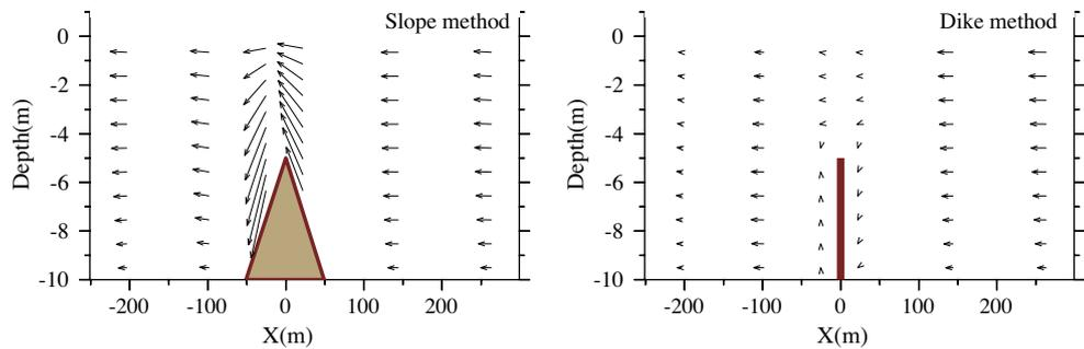
**Fig. 12.** Velocity distributions along the vertical section under slope-conforming method (left) and dike-groyne algorithm (right). The horizontal position of the vertical section is shown in Fig. 11.
