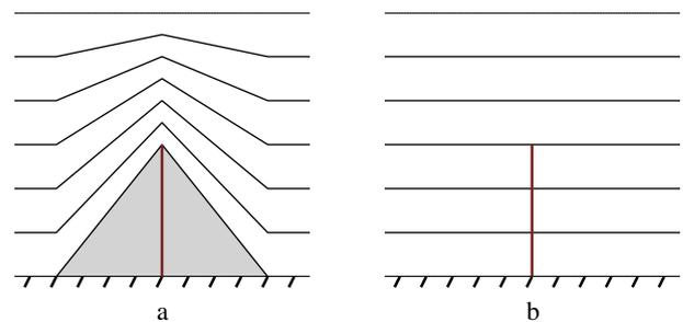
**Fig. 10.** The vertical structures of the terrain-following coordinate levels in the bed-conforming method (a) and dike-groyne treatment method (b).
