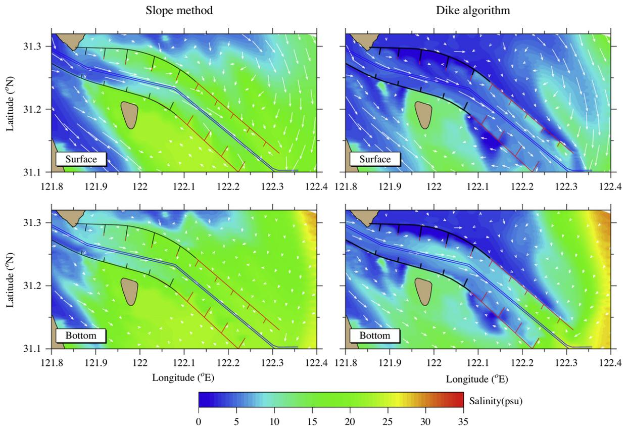
**Fig. 19.** Model-predicted distributions of the salinity near the surface (upper) and bottom (lower) at maximum ebb tide around the Deep Waterway Channel Regulation Project during spring tide of the flooding season for the cases with bed-conforming slope method (left) and dike–groyne algorithm (right).
