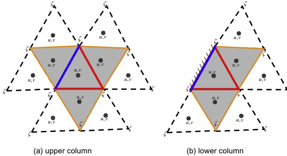
**Fig. 4.** Illustration of momentum control elements (shaded regions) used to calculate the horizontal velocity in the upper (above the height of the construction) and lower (below the height of the construction) layers.
