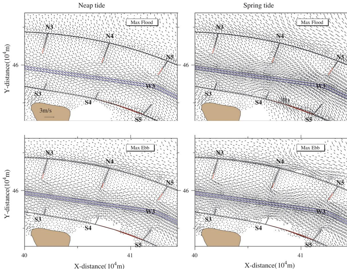
**Fig. 16.** Distributions of currents near the surface at maximum flood (upper row) and ebb (lower row) between the segments marked W2–W3 during the spring tide cycle (right column) and neap tide cycle (left column) in the flooding season predicted by FVCOM with dike–groyne algorithm.
