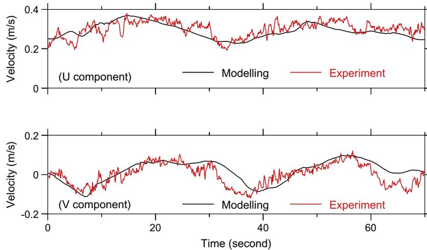
**Fig. 8.** The model-data comparison of  $u$  and  $v$  components of the fluid velocity at point #3 for Exp#1 under a submerged groyne condition. Red lines indicate the time series of the measured velocity recorded in the laboratory experiment and black lines are the model-computed velocity. (For interpretation of the references to color in this figure legend, the reader is referred to the web version of this article.)
