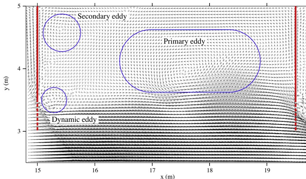
**Fig. 7.** Snapshot of simulated flow patterns in the fourth groyne field for Exp#1 under an emerged groyne condition. Solid red lines indicate emerged groynes, and dashed red lines indicate the submerged slope edges of groynes. Blue cycles show the locations of primary, secondary and dynamic eddies. (For interpretation of the references to color in this figure legend, the reader is referred to the web version of this article.)
