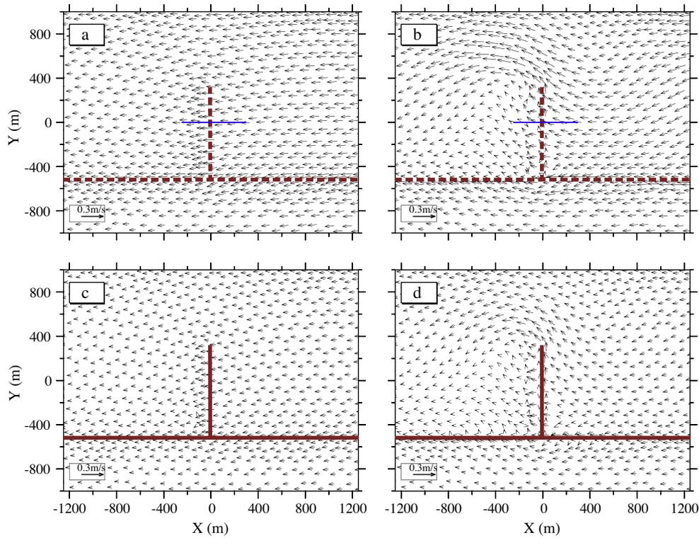
**Fig. 11.** Distributions of horizontal currents near the surface (upper row) and bottom (lower row) for the idealized estuary case driven by tidal forcing with slope bed-conforming method (left column) and the dike-groyne algorithm (right column). The blue solid lines in the upper row panels indicate the location of the velocity sections shown in Fig. 12. (For interpretation of the references to color in this figure legend, the reader is referred to the web version of this article.)
