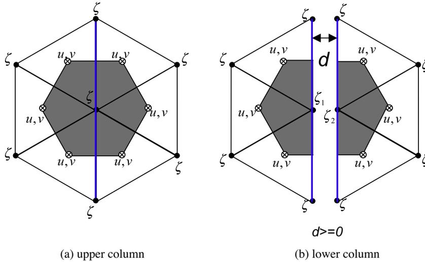
Fig. 2. Sketch of the separation of the control element at dikes or groynes. The shaded regions indicate the tracer control elements (TCEs).
